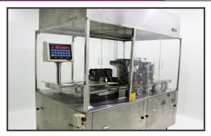
The sterile production facilities must be free of airborne particles that should not exceed 100 in number per cubic feet area for class 100 clean room (FS-209E). This is essential for sterile production. The clean room is maintained by HEPA filter & laminar air flow.
